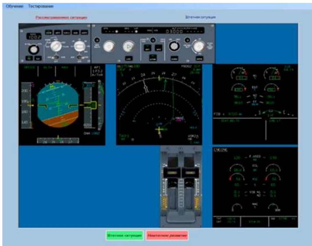
Fig. 2 Dynamic image on the monitor screen when deviations in flight parameters from the normal mode begin
